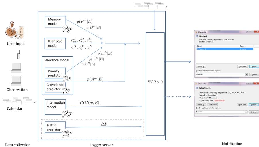
Figure 1: Jogger system components. Two interfaces of the system are presented on the right, one for the original system architecture (marked with straight arrow) and one that includes consideration of traffic-sensitive travel to a meeting (dashed arrow).
